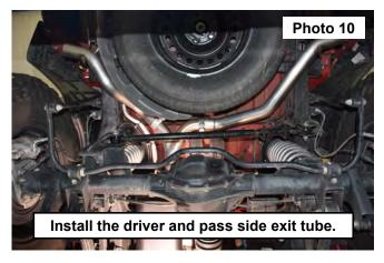
10. Remove the driver side hanger mount from the frame. Then place it onto the exit tube mount and re-install onto the frame using the OE hardware and a 15mm socket. See Photos 11 and 12.
